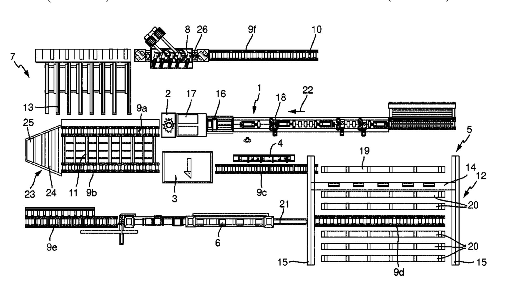
tively, the pilger rolling mill, the first buffer, the annealing furnace, the second buffer and the straightening machine.
