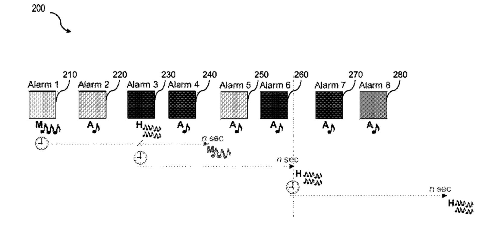
highest priority grade alarm condition are conveyed at a second level, the second level being different from the first level.
