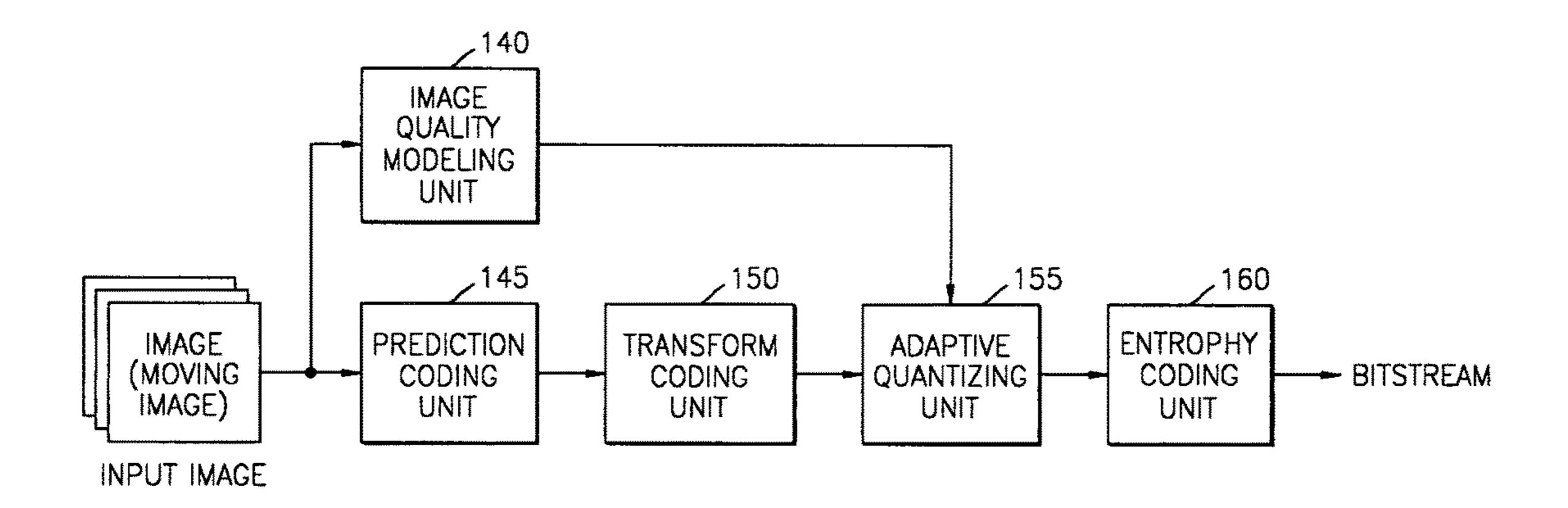
bution, (c) quantizing image data in accordance with the quantization parameter, and (d) coding entropy of the quantized image data.
