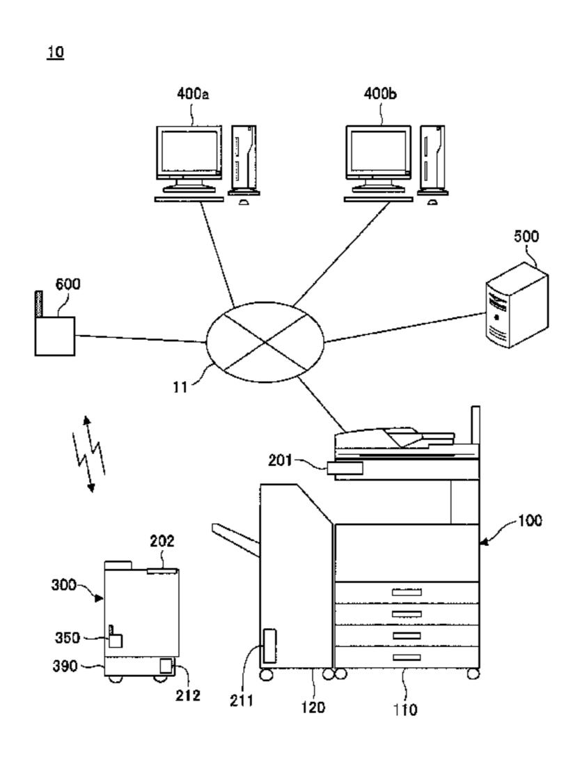
apparatus to generate the printed matter based on the print job authenticated by the delivery authentication processing unit and to output the printed matter to the printed matter delivery apparatus; and a receipt confirmation unit obtaining receipt information input into the printed matter delivery apparatus at a delivery destination.
