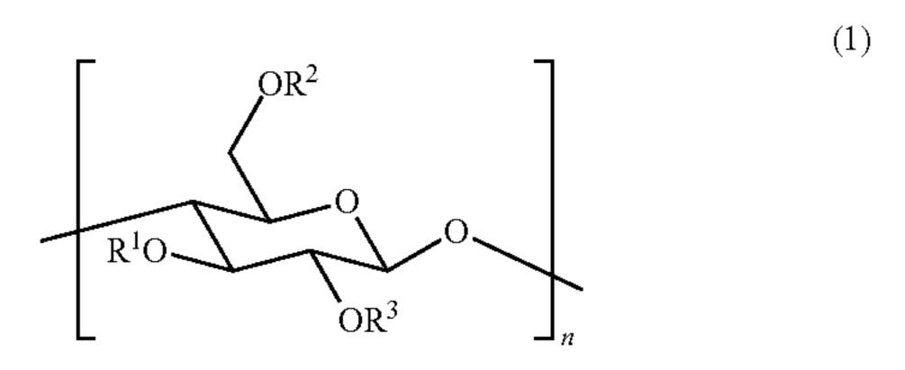
R<sup>1</sup>, R<sup>2</sup>, and R<sup>3</sup> in the formula (1) each independently represent a hydrogen atom or an acyl group. n represents an integer of 2 or greater. However, at least one of n numbers of R<sup>1</sup>s, n numbers of R<sup>2</sup>s, or n numbers of R<sup>3</sup>s represents an acyl group.
