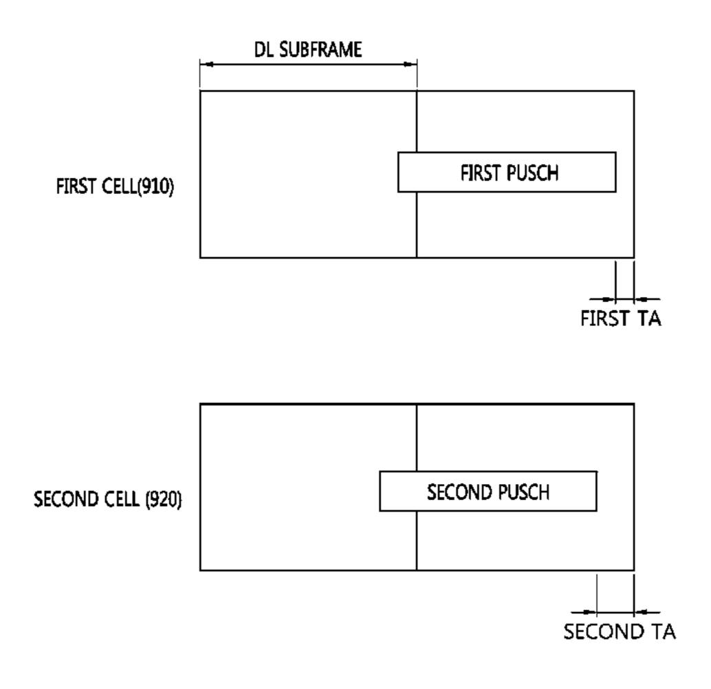
configured so that an uplink can be always transmitted regardless of the timing difference.
