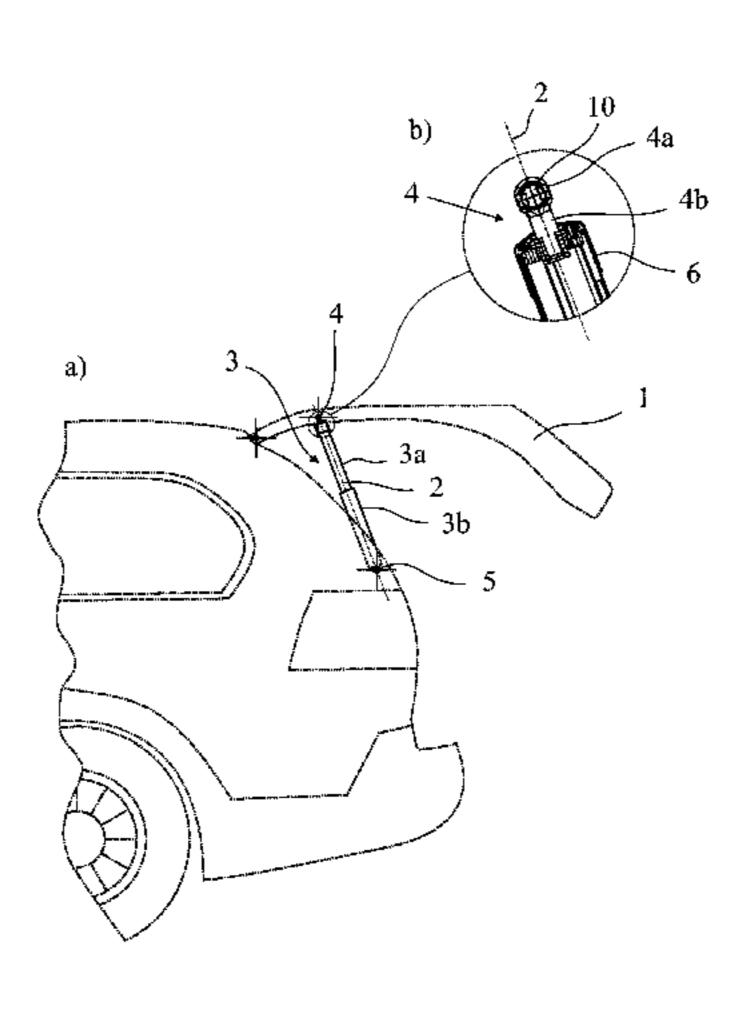
of the sealing opening is elastically deformed by the engagement with the connection head and is therefore widened, and that the peripheral region of the sealing opening is subsequently deformed back elastically in frictionally sealing engagement with the connection neck.
