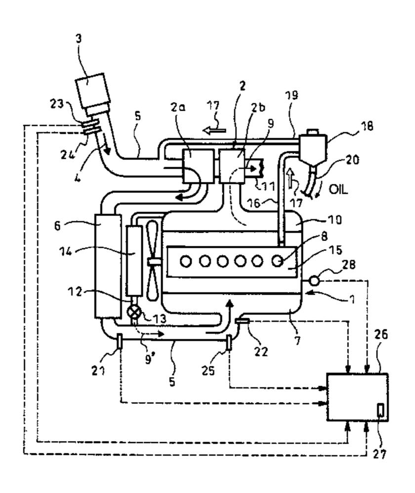
gence in a last determination is compared with a current divergence; if difference between the divergences is beyond a predetermined range, the gas return pipe 19 is determined to be in disconnection from the intake pipe 5.
