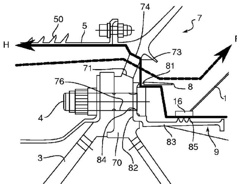
towards the outside, each discharge opening being radially aligned with a connecting segment of the main body to allow each flow of oil to be discharged radially between the airflows.
