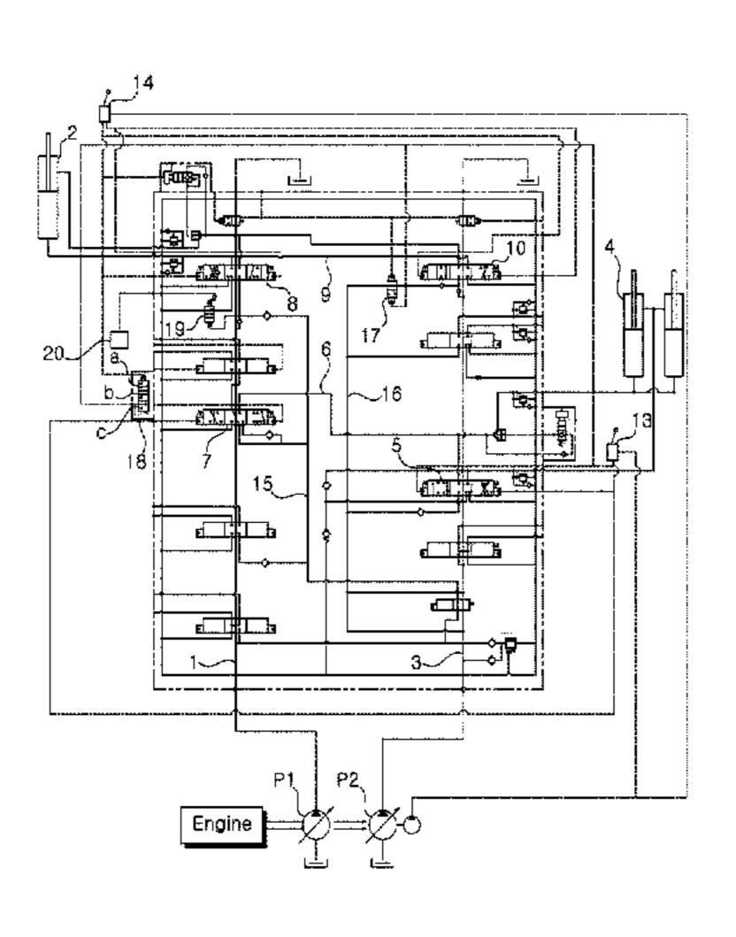
is disposed in the flow path between the working fluid inlet port of the first arm control valve and a hydraulic tank; and a second boom control valve spool having a parallel pressure section in which the boom-up pilot pressure does not increase with respect to the boom-up strokes during the simultaneous boom-up and arm-in operation.
