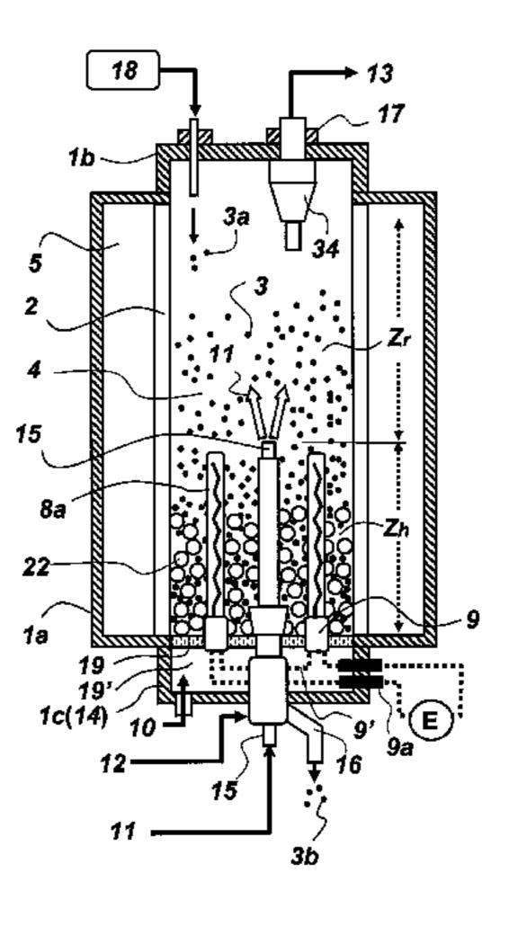
gas at such a rate that the silicon particles can be intermixed between the reaction zone and the heating zone in a continuous, fluidized state.
