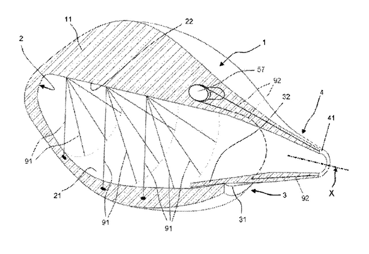
to the dorsal wall, thereby causing a pulsed ejection of a propeller jet from the chamber through the outlet opening.
