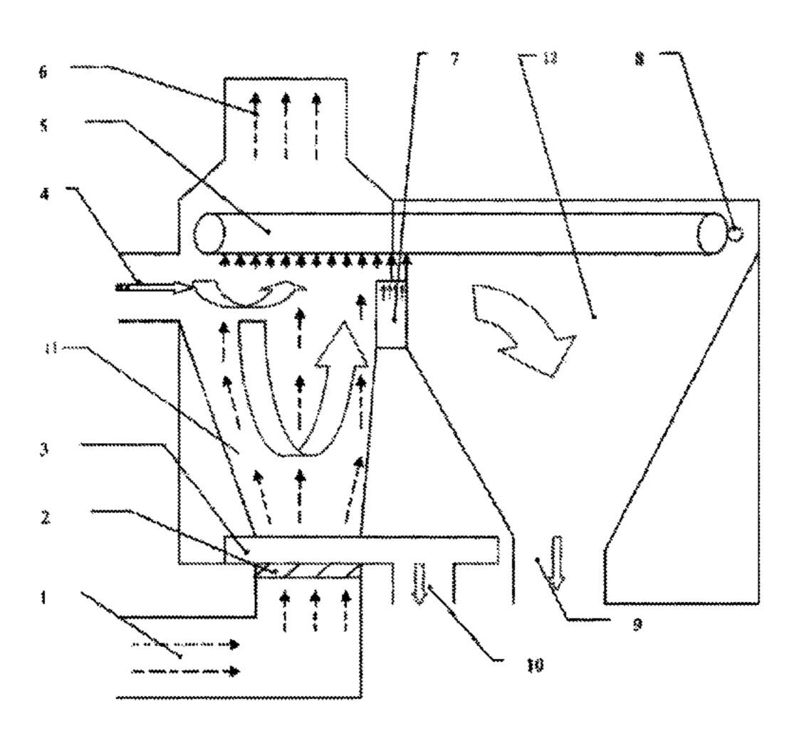
side of the end of the belt conveyer, a vibration trough is arranged at the lower part of the separation silo, a damper plate is disposed underside thereof, an air inlet is located underbelly thereof at the bottom of the separation silo, a rejection outlet is installed at the underside end of the vibrating trough.
