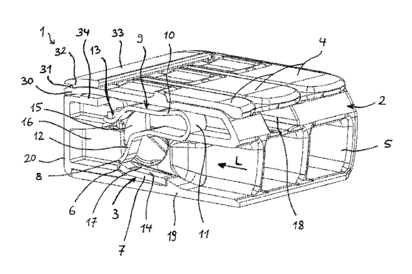
be clamped. The busbar (7) has a groove-like recess (14) in the conductor insertion direction (L) upstream of the clamping location adjacent to the clamping edge (6).
