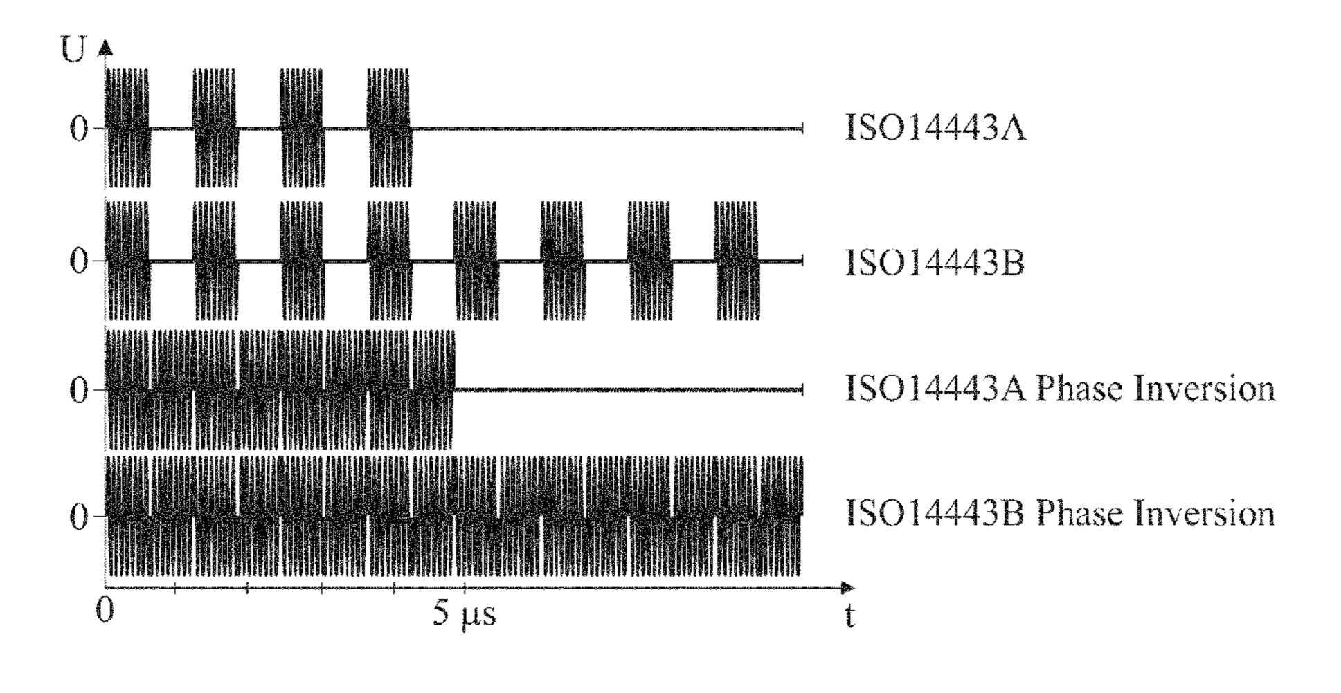
B by inverting a phase at transitions between said half-periods. Said synchronizing is carried out although no time window without a tag transmitting exists within the transmitted data frame.
