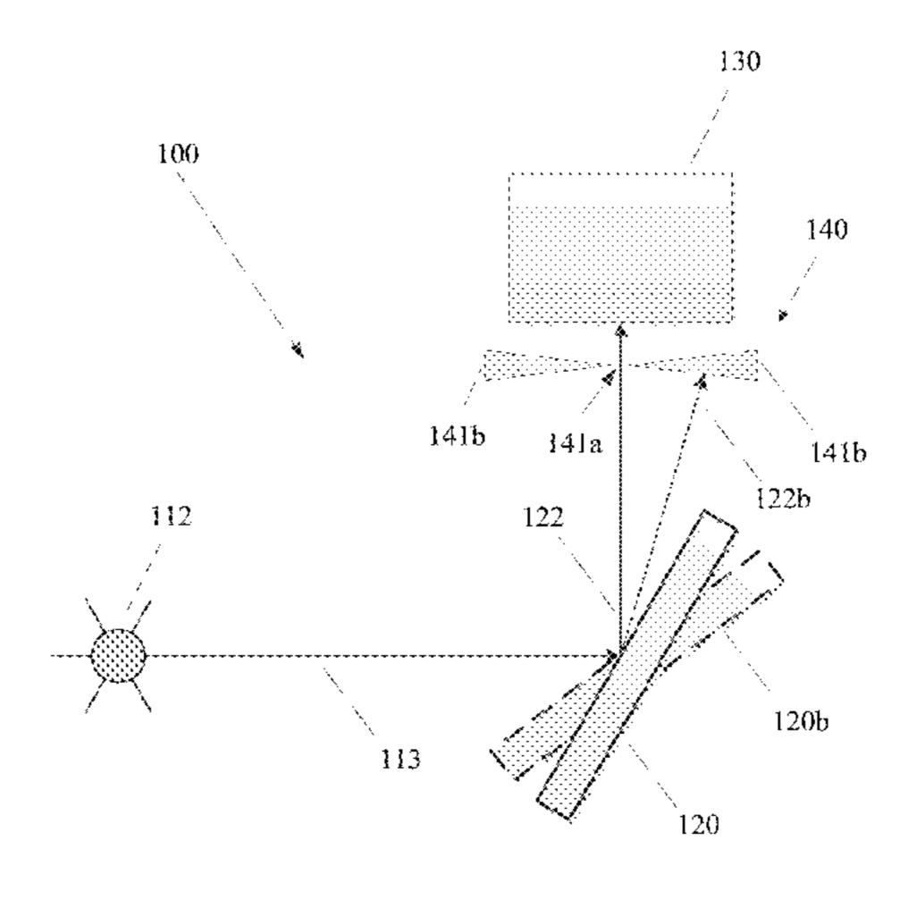
position causing the light beam to be blocked by the aperture. The optical device may be configured to operate as a shutter, chopper, modulator and/or deflector.
