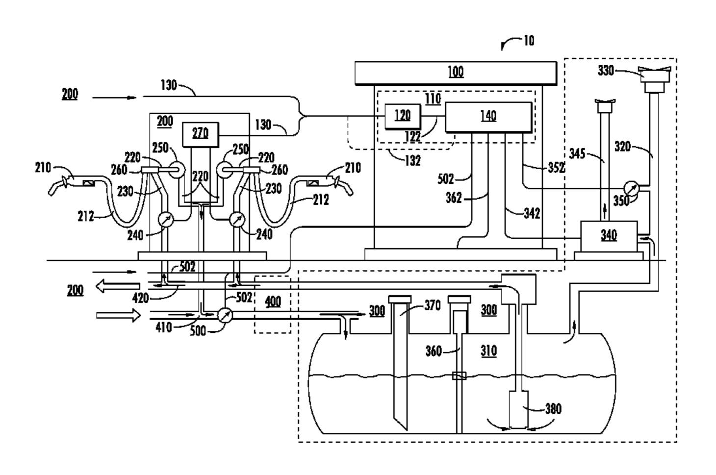
methods and apparatus also provide for the determination of fuel dispensing system vapor containment integrity, and the differentiation of true vapor recovery failures as opposed to false failures resulting from the refueling of vehicles provided with onboard vapor recovery systems.
