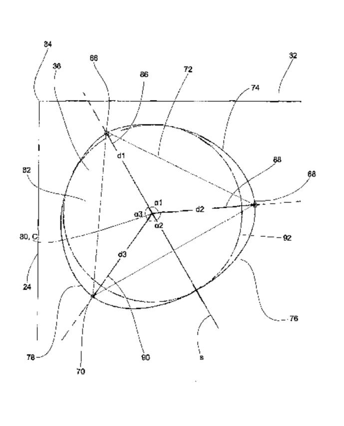
the same number of thoroughly curved lines connecting the corner points. The corner points include first, second and third corner points.
