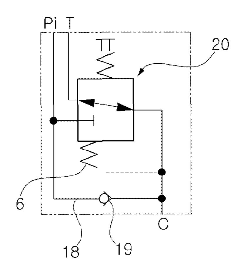
elastically supports the spool so as to communicate the secondary pilot pressure port and the tank port with each other; and a check poppet that is disposed in an openable and closable manner at a pilot passage whose inlet side communicates with the secondary pilot pressure port and whose outlet side communicates with the port of the pilot pump.
