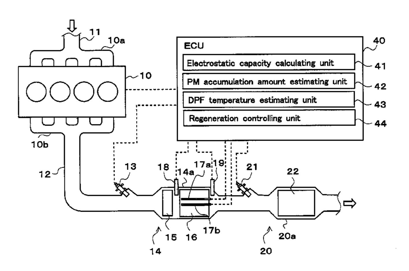
when the inside temperature is at or above the SCR activation temperature, and executes the forced regeneration with another amount of fuel supplied for causing the inside temperature to reach the upper limit temperature, when the inside temperature is below the SCR activation temperature.
