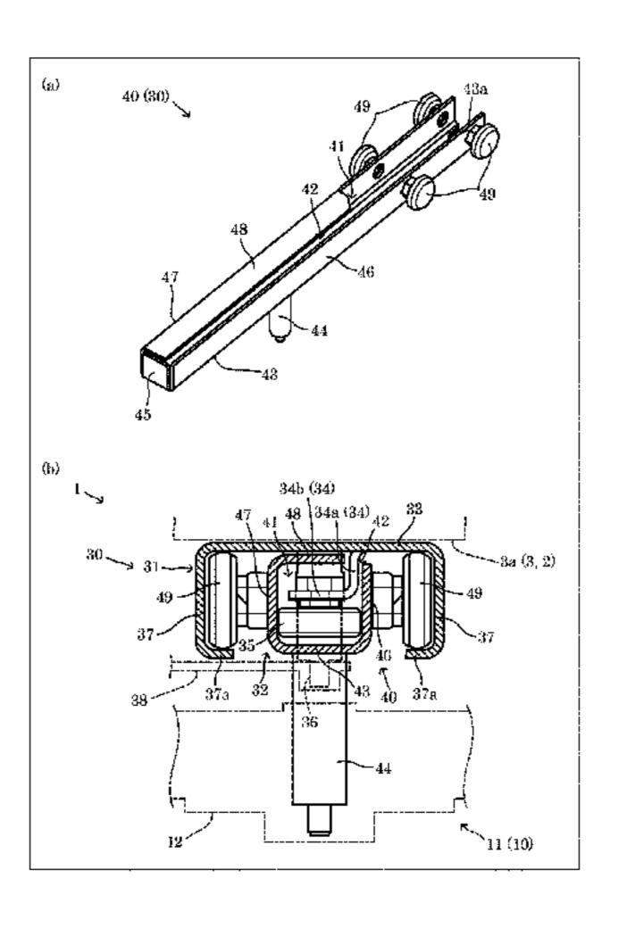
define a receiving groove for receiving the guide body; and a top wall that forms a slit opening for receiving the holding section.
