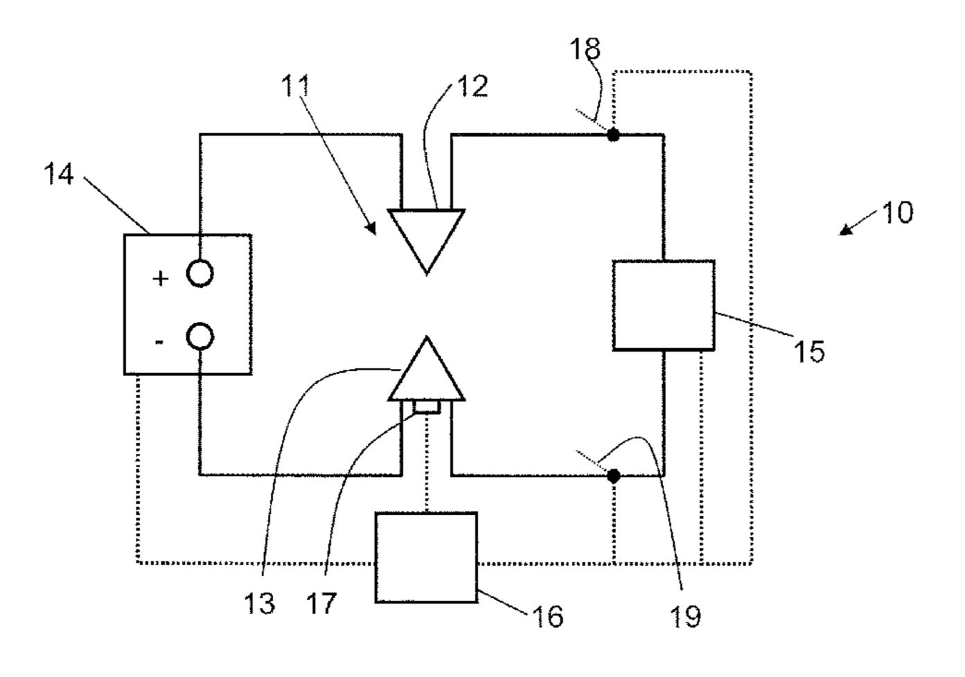
recognizing an effected ignition (at the point in time  $t_Z$ ) of the plasma, the voltage is reduced between the anode and the cathode to a maintenance voltage  $(U_A)$ .
