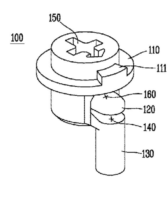
The first stopper is fitted into and fixed to the plurality of fitting grooves according to the rotation of the dial.
