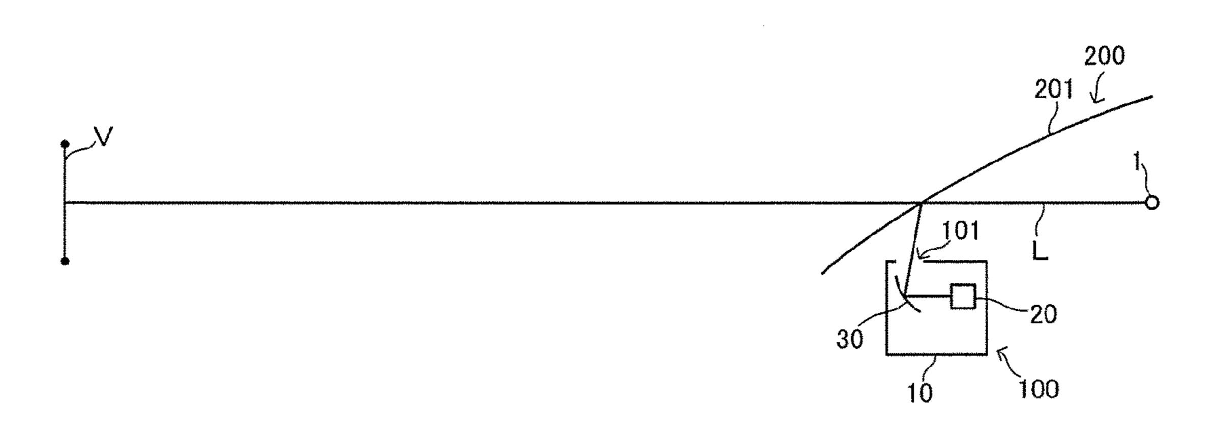
and adjusts the projection location of display light (L) on front glass depending on the height of the observer's point of view.
