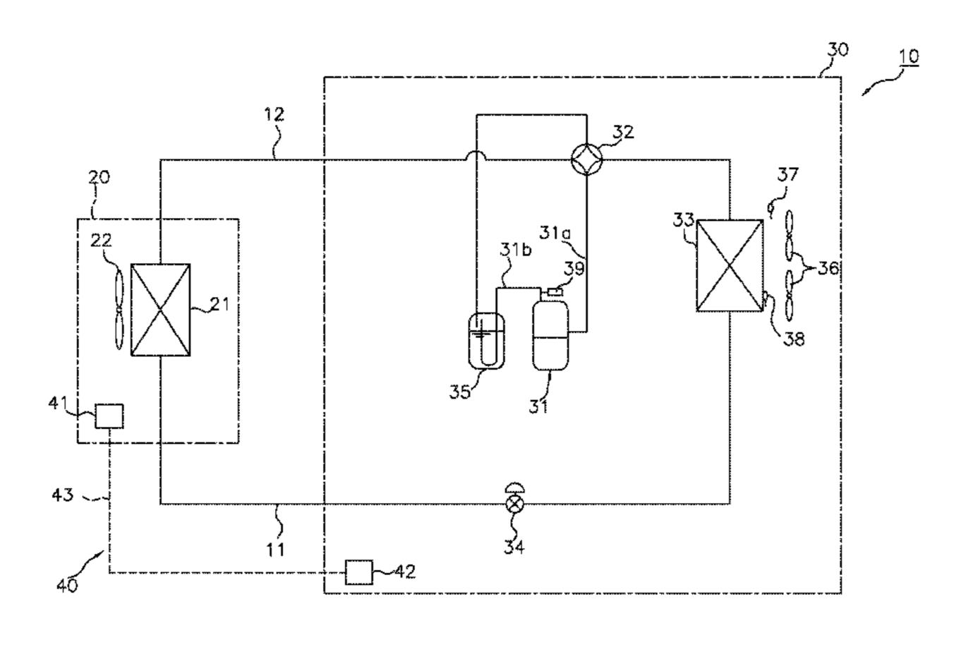
fan is determined using a corrected converted high pressure value. The corrected converted high pressure value is obtained by correcting the current converted high pressure value based on the past converted high pressure value.
