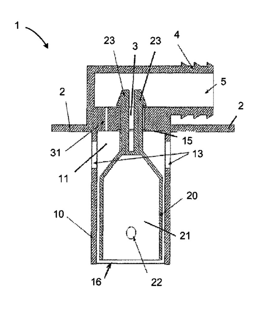
of which the valve body (20) is held movably in the valve housing (10).
