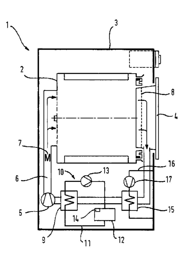
ture can be conducted in a respective closed circuit through the associated heat exchanger for an exchange of heat with the working medium, and the substance mixture circulates between the associated heat exchanger and at least one reservoir in the respective closed circuit. The reservoir can be refilled layer-by-layer with the substance mixture conducted through the respective associated heat exchanger.
