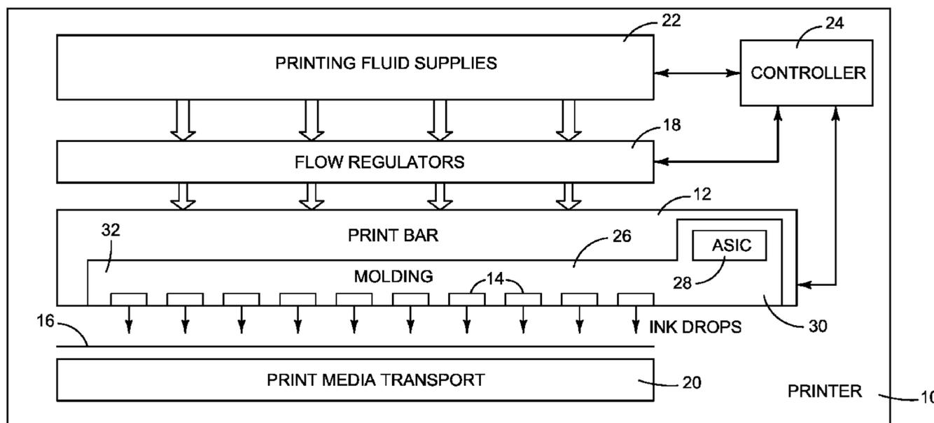
molding except at the channel. The assembly further comprises a first external electrical contact electrically connected to the fluid dispensing die and exposed outside the molding to connect to circuitry external to the assembly, and a non-fluid dispensing die electronic device buried in the molding and electrically connected to the first external electrical contact.
