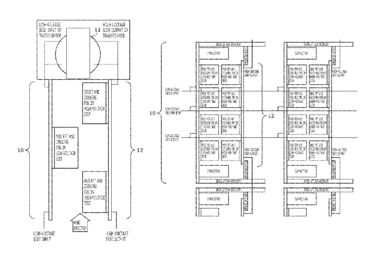
which two input and output substrates are opposed and are connected by insulation members, and another wind-tunnel structure arranged in the downstream of the wind-tunnel structure and including the LLC resonant structure therein. The wind-tunnel structures are integrated with each other.
