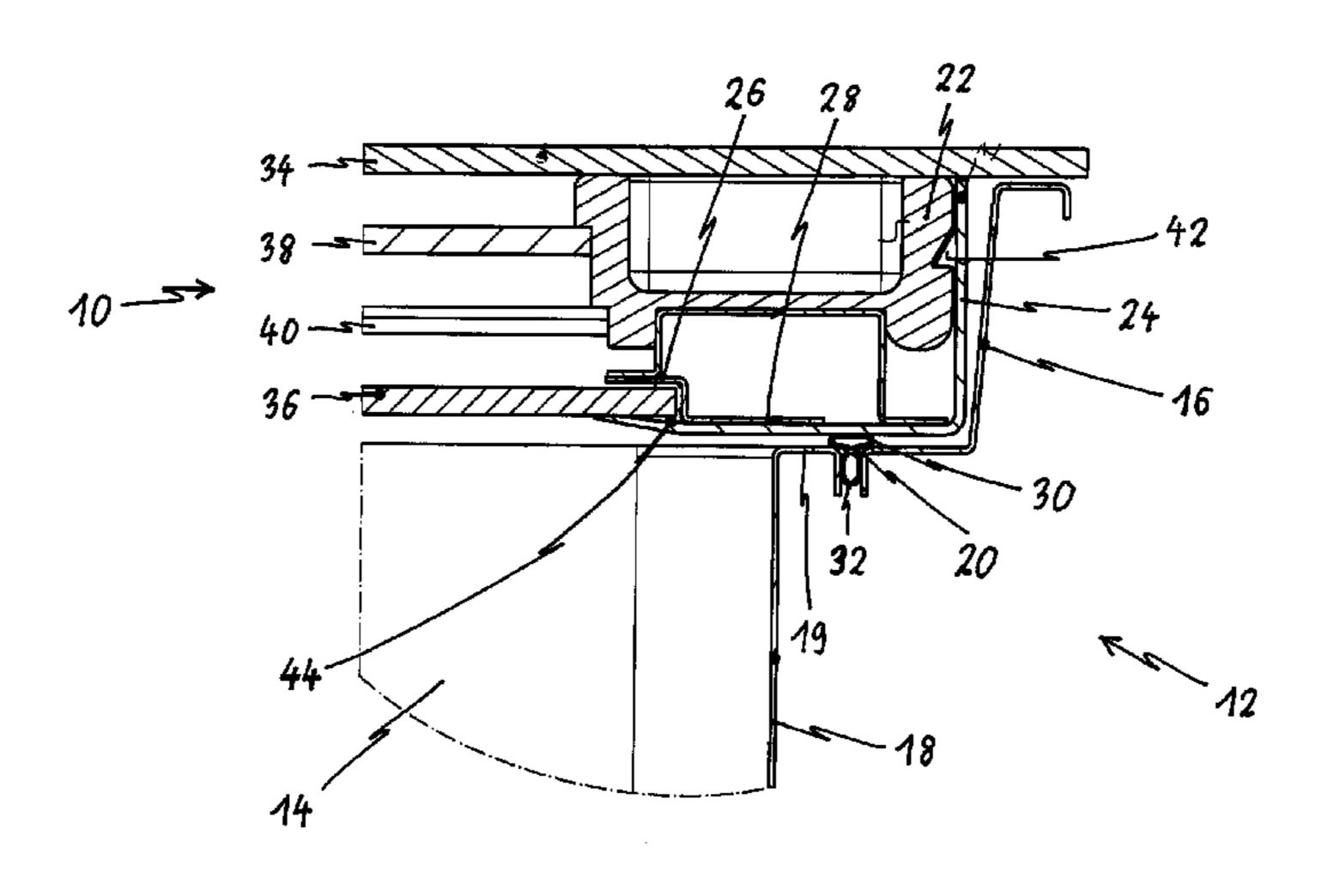
choke. A sealing element made of a high temperature resistant textile material is arranged between the cover element and the inner glass panel. A corresponding chassis is provided for the oven or the appliance.
