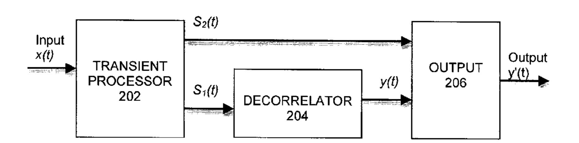
signal into at least two components, in which the first component is characterized by fast fluctuations in the input signal envelope, and a second component that is relatively stationary over time; processing the second, stationary component by a decorrelation circuit; and constructing an output signal by combining the output of the decorrelator circuit with the input signal and/or the first component signal.
