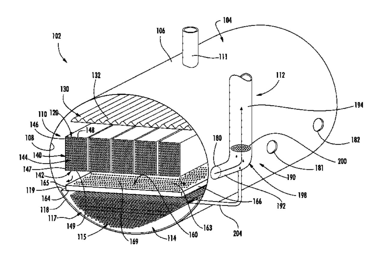
another so as to define one or more vapor passages. A refrigerant distributor is positioned above the tube channel. The refrigerant distributor delivers a refrigerant onto the plurality or tubes toward the refrigerant pool zone.
