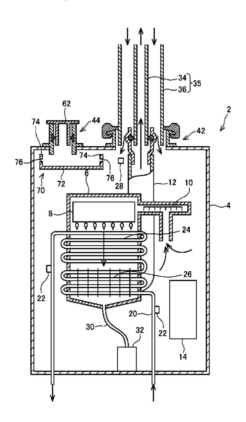
closed, whereas in a case where it is installed in the separate-pipe system, the air supply passage of the air supply/exhaust port is closed. The combustion apparatus includes: a supplied-air temperature sensor; and a guide member, which is located near the air supply passage of the air supply/exhaust port or the air supply passage of the air supply port, and by which air flowing into the space in the housing is guided to the supplied-air temperature sensor.
