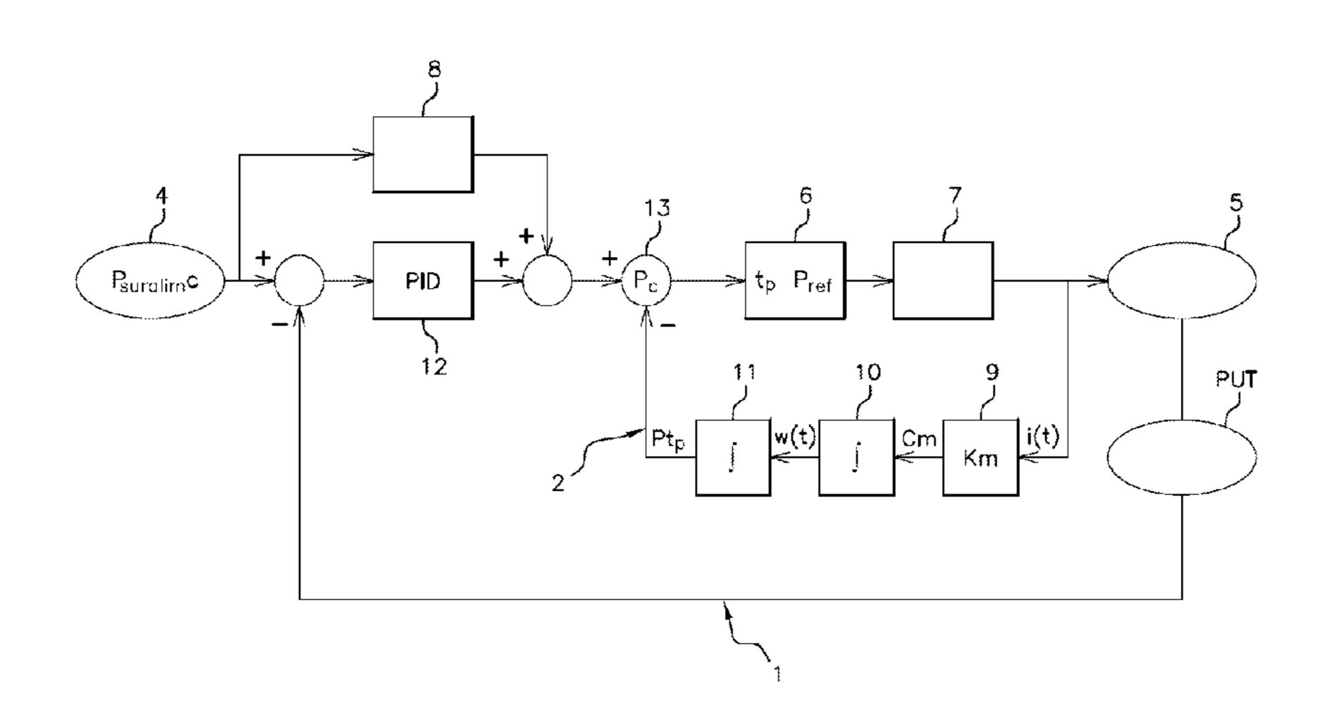
obtaining the position reached by the wastegate at the end of the monitoring time by integration of the speed; comparing the position reached with the set position; and repeating the method until the set position is reached.
