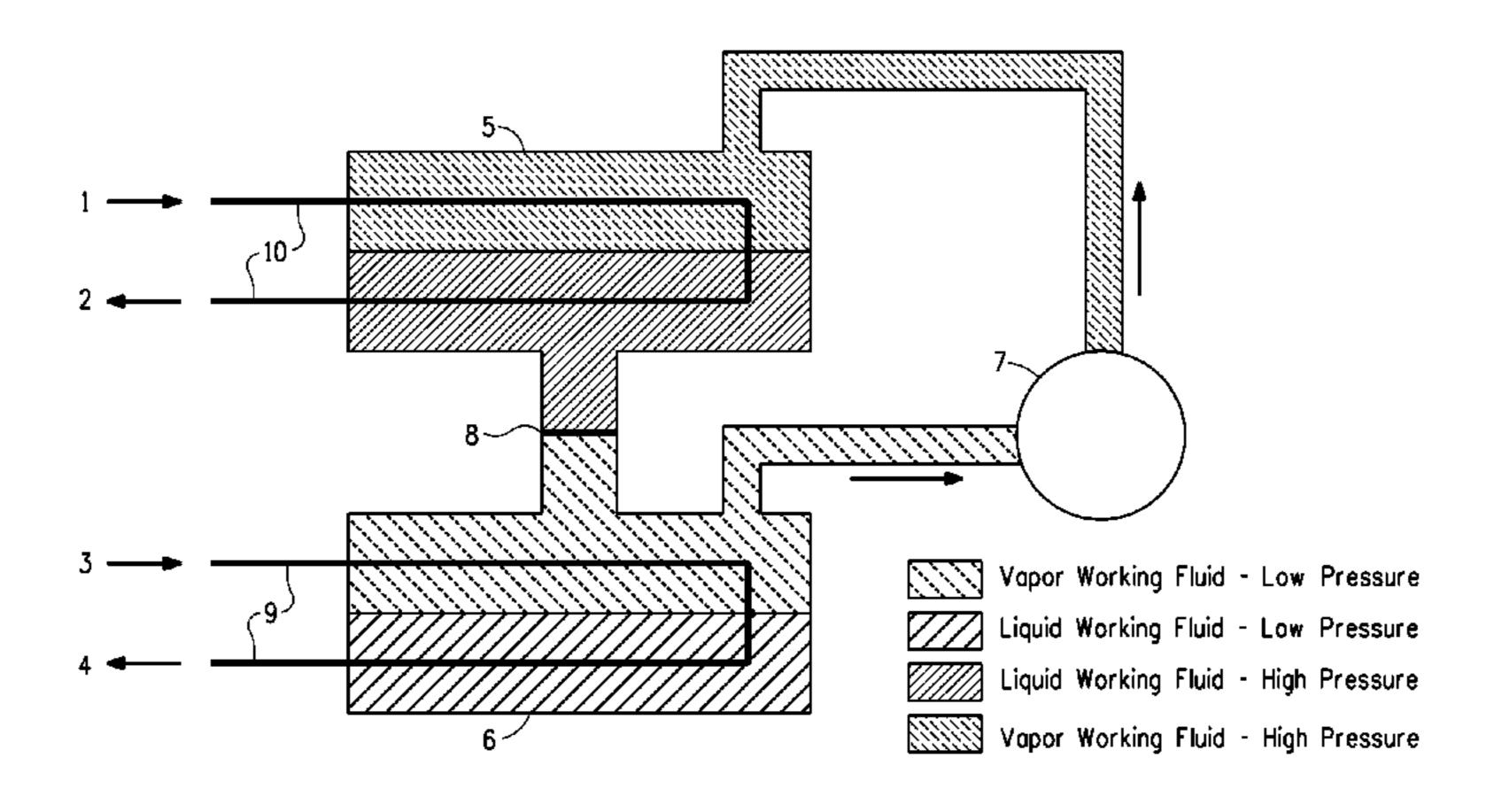
Also disclosed herein is a high temperature heat pump apparatus containing a working fluid comprising Z-1,1,1,4, 4,4-hexafluoro-2-butene.
