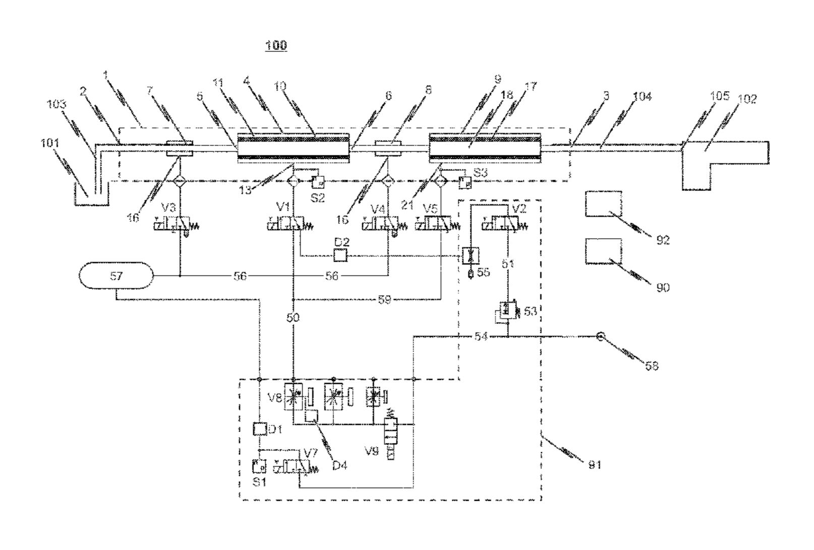
to the powder inlet valve or the powder outlet valve per time unit when the actuation pressure is adjusted and maintained. An evaluation device compares at least one detected or determined gas flow value with a corresponding set value and automatically generates an error and/or alarm signal when a deviation is detected.
