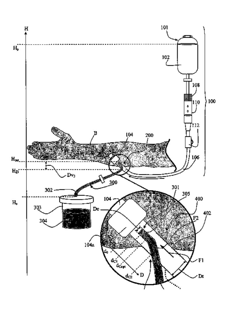
perfusion catheter (104), in the direction of flow (F1) of the perfusion product (102), from a perfusion product reservoir (101) towards the perfusion catheter (104).
