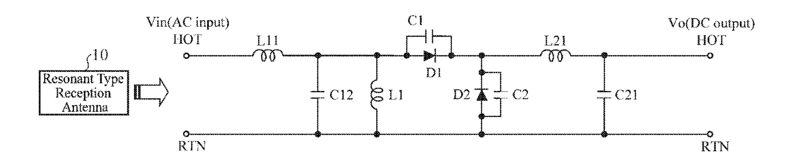
circuit that smooths the voltage rectified by the current doubler rectifier circuit into a direct voltage.
