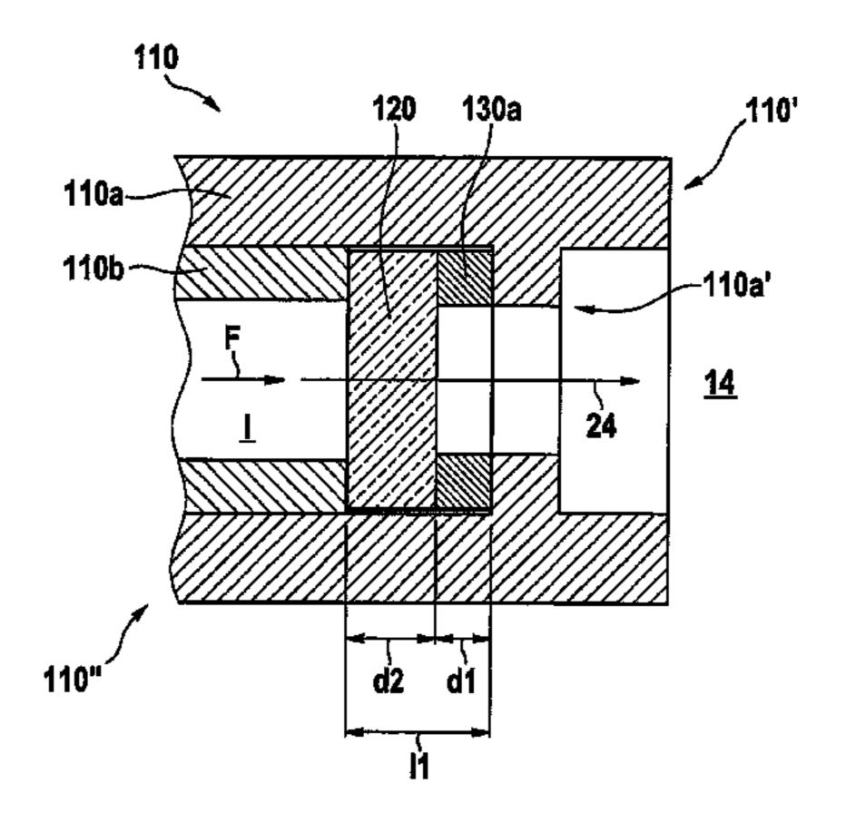
engine; the casing including at least one casing part and a combustion chamber window joined to the casing part to form a seal at least regionally; characterized in that at least one sealing element, whose coefficient of thermal expansion at an operating temperature of the laser spark plug is greater than the coefficient of thermal expansion of the casing part at the operating temperature of the laser spark plug, is provided between the casing part and the combustion chamber window.
