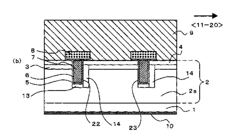
in a <0001> direction with respect to a plane parallel to the <0001> direction. The insulated gate silicon carbide semiconductor device can relieve an electric field of a gate insulating film and suppress an increase in on-resistance and provide a method for manufacturing the same.
