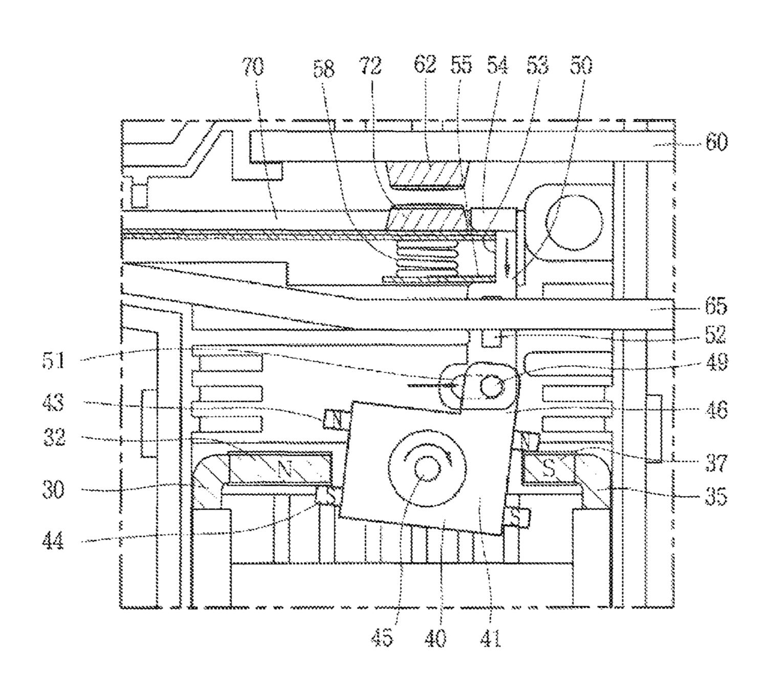
transmission lever, and an elastic member providing contact force such that the movable contactor is brought into contact with the first fixed contactor or separated from the first fixed contactor, while moving according to a movement of the transmission lever.
