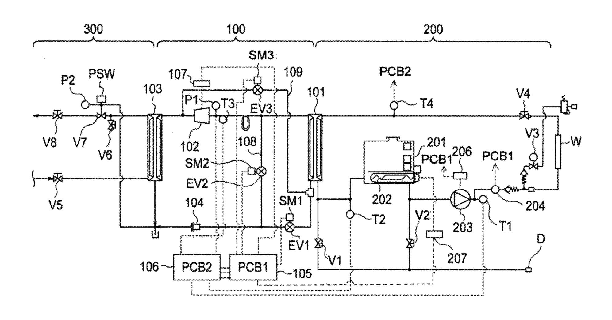
the work temperature detected by a first sensor, and PCB1 controls opening and closing of an electronic expansion valve by driving a stepping-motor according to a pulse signal generated based on result, and controls flow rate of refrigerant.
