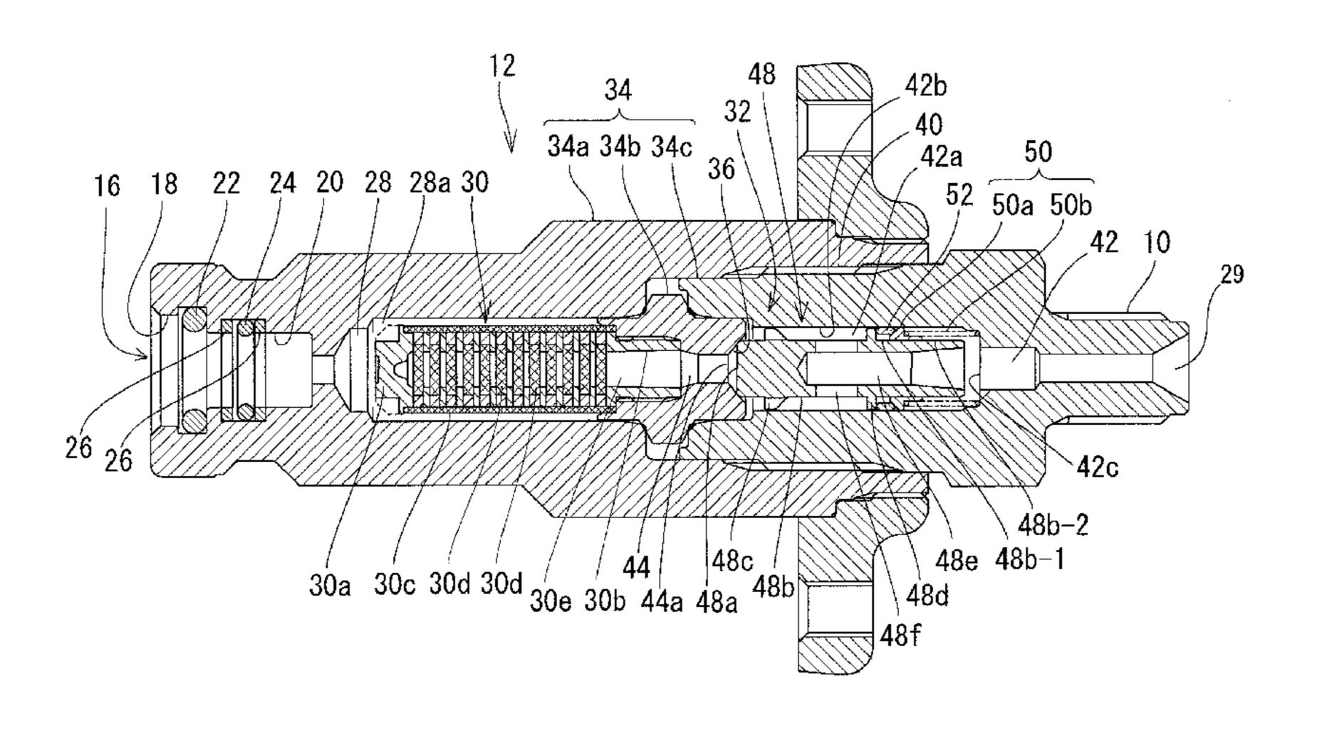
displaced upstream and downstream, and an urging member support portion supporting an urging member urged upstream so that the urging member urges the sliding resistance imparting member upstream, thereby causing the sliding resistance imparting member to increase in outer diameter while being arrested by the arresting portion.
