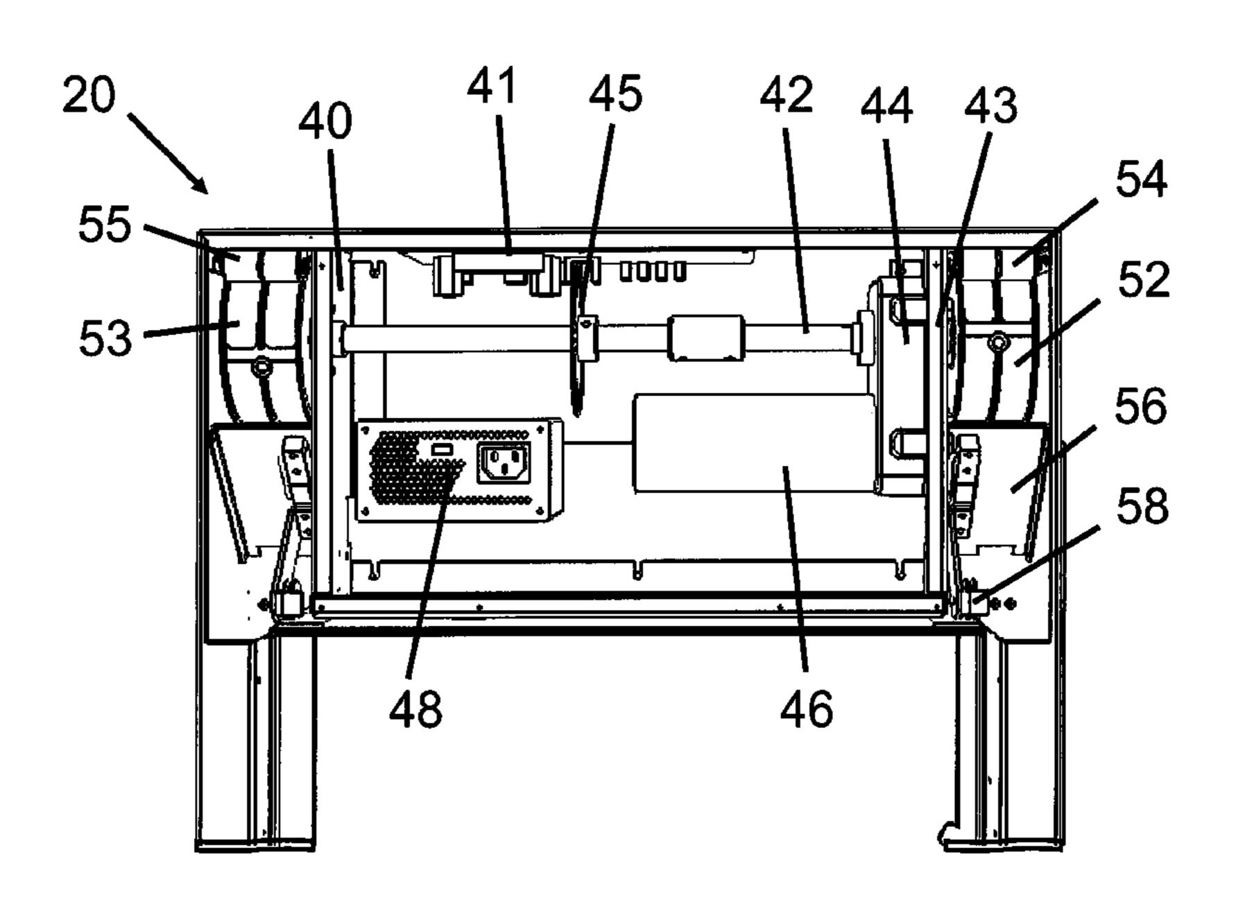
one load sensor, wherein the control circuit controls operation of the motor responsive to the load signal. The control circuit causes the platform to travel upward by driving the motor to rotate the shaft in a first direction to wind the lift tethers onto the respective lift drums and causes the platform to travel downward by driving the motor to rotate the shaft in a second direction to unwind the lift tethers from the respective lift drums.
