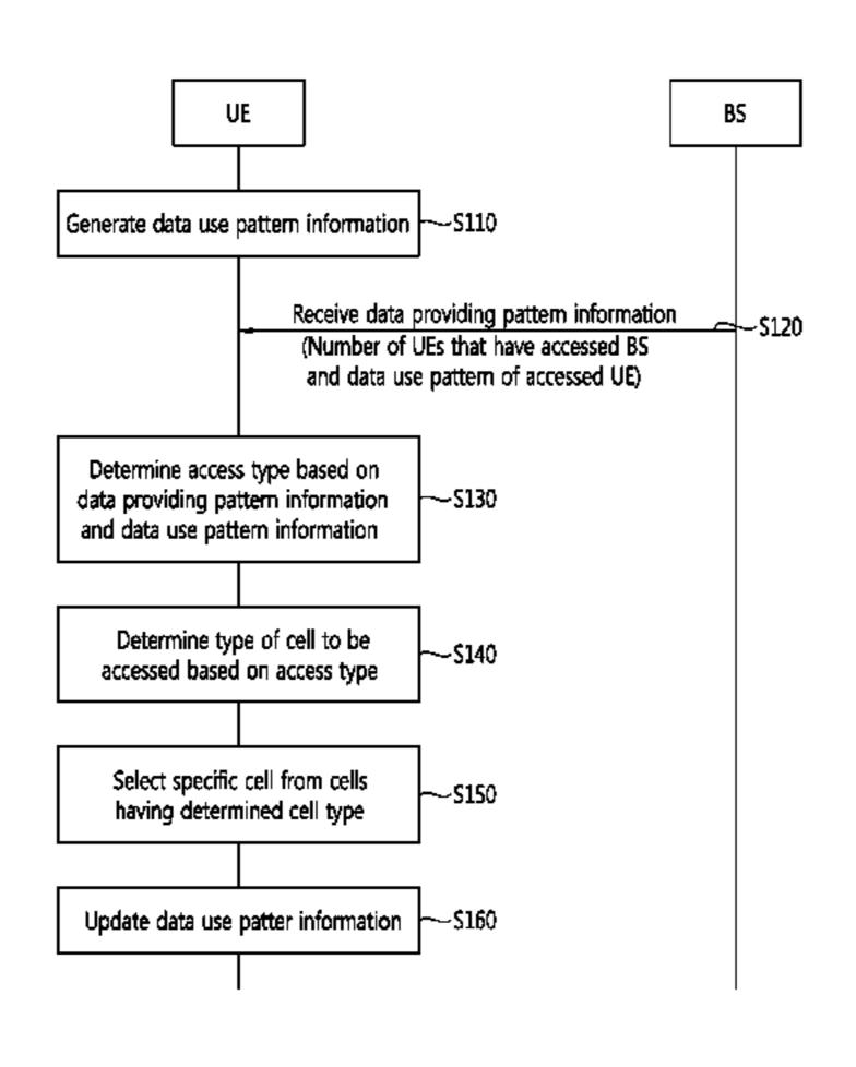
data provided by the wireless communication system for each specific moving speed of the UE, determining an access type of the UE based on the data use pattern information and the data providing pattern information, selecting a type of a cell to be accessed according to the access type and selecting a cell from cells having the cell type.
