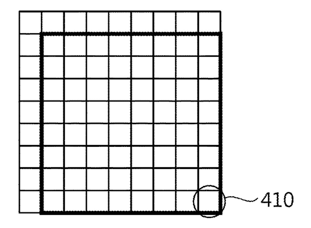
Step2. Interpolate right most and bottom samples (S420)
