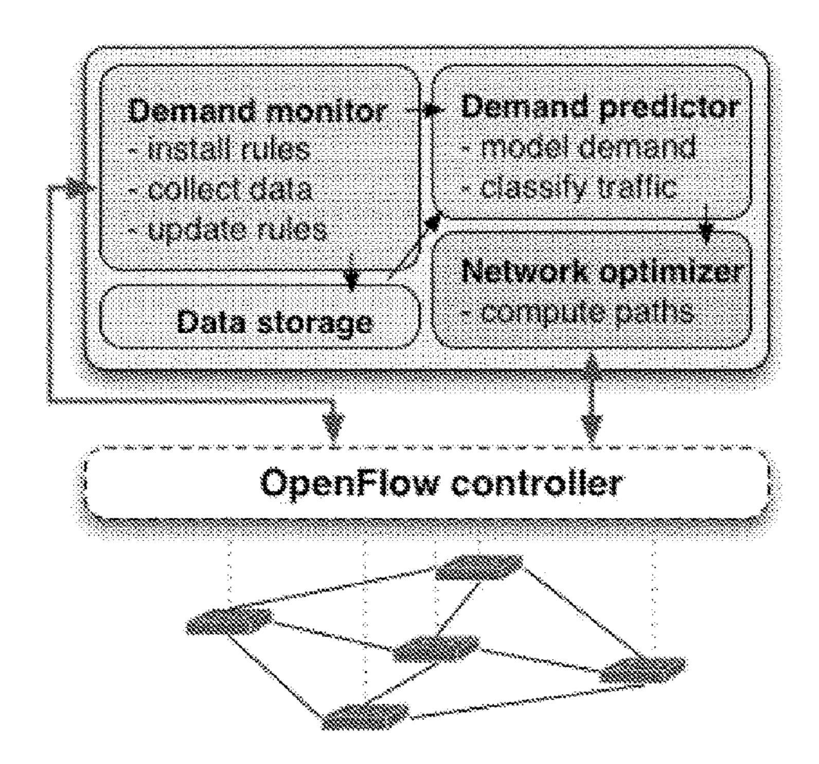
The system architecture is illustrated above and consists of four major components:1) application demand monitor, 2) storage for monitoring data, 3) application demand predictor, and 4) network optimizer. We describe each component below:
