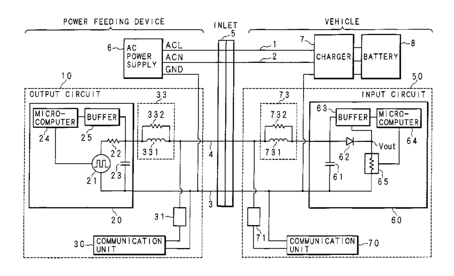
the input circuit via a bandpass filter. A low-pass filter is interposed between the output circuit and the communication unit. A low-pass filter is interposed between the input circuit and the communication unit.
