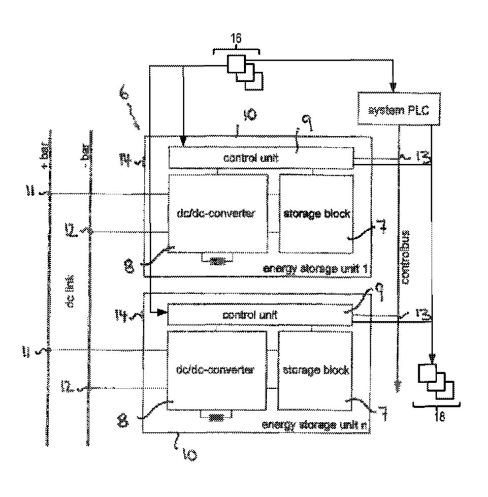
whose outer side two connections are provided for connecting to the DC voltage circuit.
