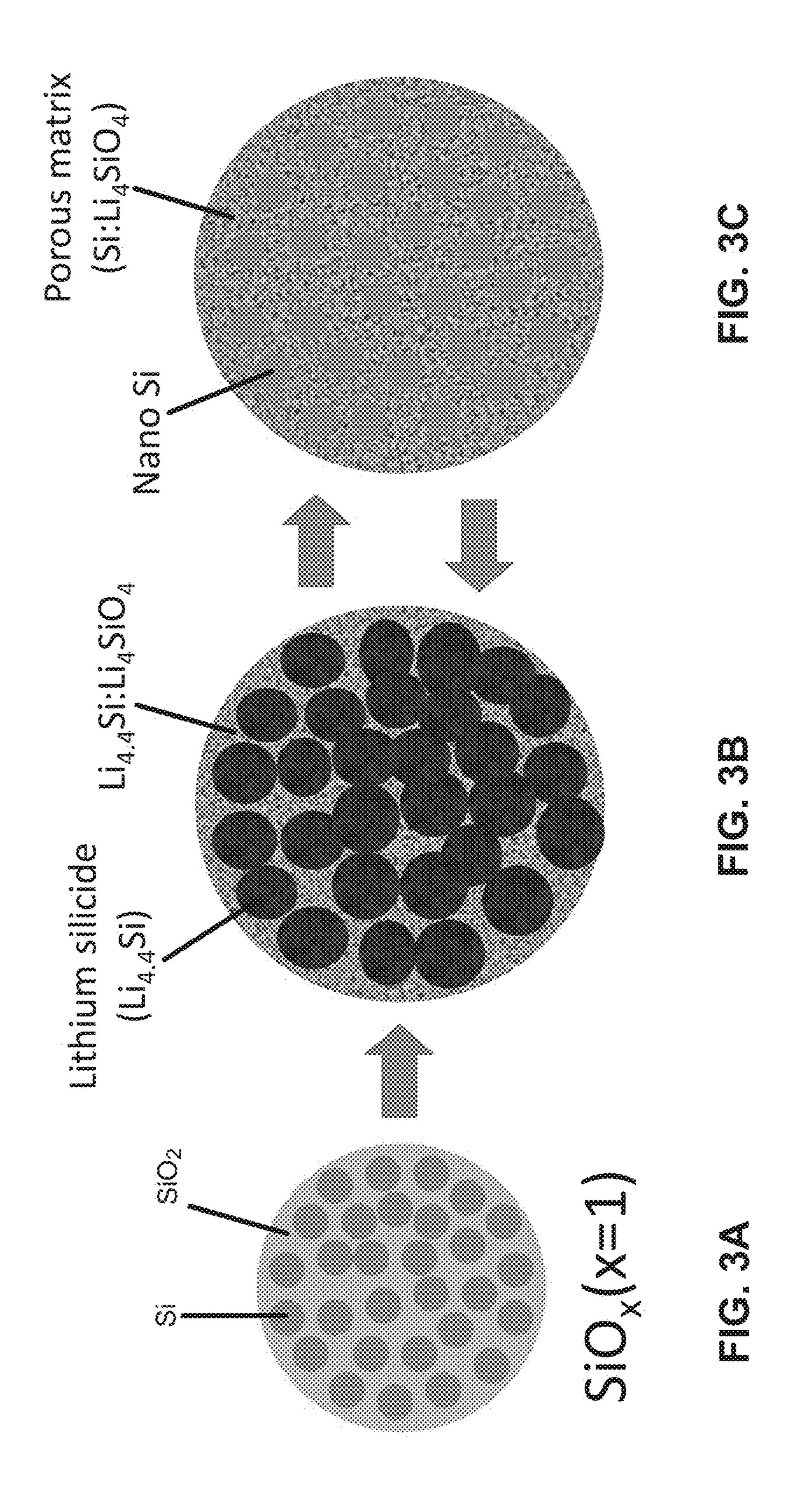
SILICON-SILICON OXIDE-LITHIUM COMPOSITE MATERIAL HAVING NANO SILICON PARTICLES EMBEDDED IN A SILICON:SILICON LITHIUM SILICATE COMPOSITE MATRIX, AND A PROCESS FOR MANUFACTURE THEREOF
